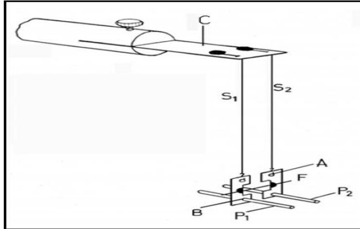
Figure 2. Schematic of the instrument for measuring bending rigidity
