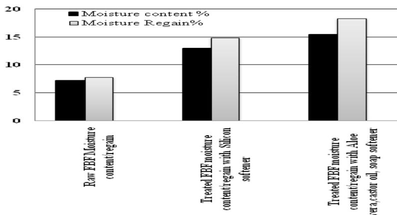
**Figure 4.** Comparison of moisture content and regain of raw and treated FBF.
