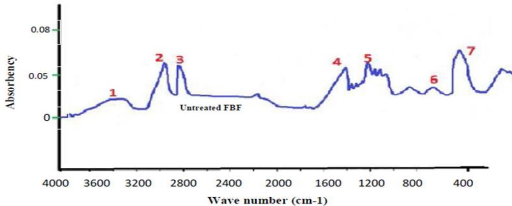
Figure 5. Infrared spectroscopy of false banana fibers
