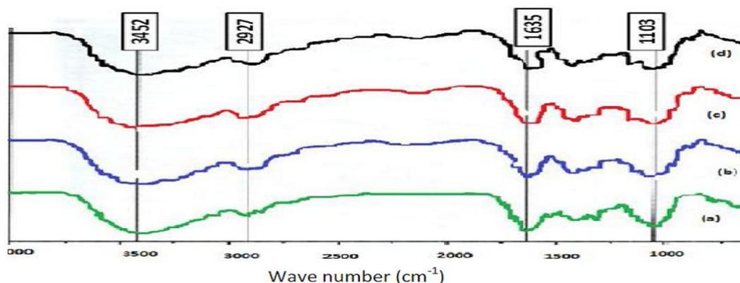
**Figure 6.** FTIR of FBF (a) raw fibers (b) treated with 2.5% (c) treated with 5% and (d) treated with 10% of NaOH
