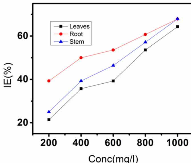
**Figure2.** Variation of inhibition efficiency against concentration of *D. tripetela* extract(leave, root and stem)
