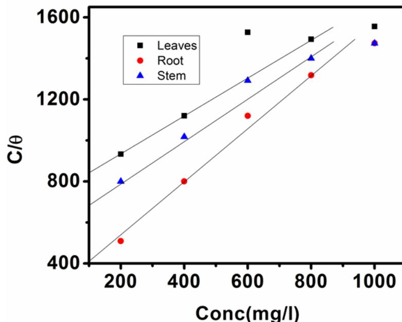
Figure 3. Adsorption isotherms for leaf, stem and root extracts of *D. Tripetela*
