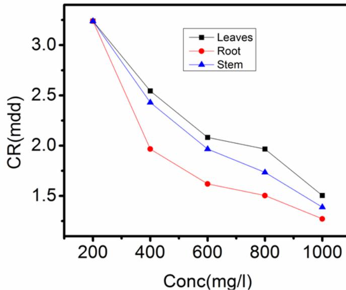
Figure 1: Corrosion rate of mild steel with concentrations of *D. Tripetela* extract.
