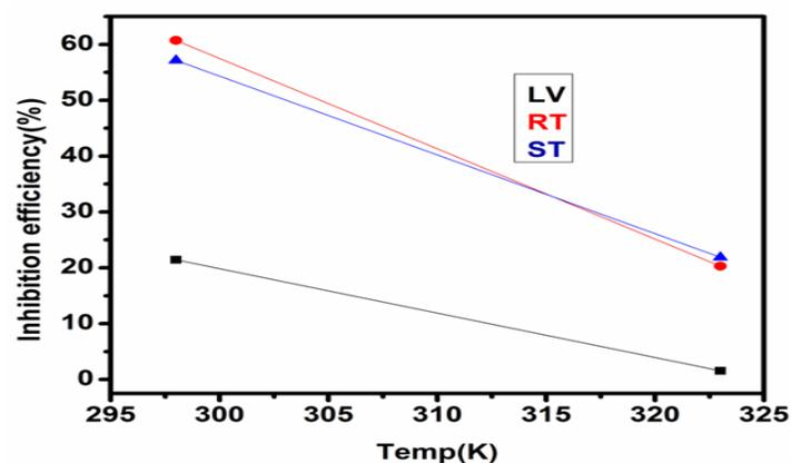
Figure 4: Variation of inhibition efficiency against temperature
