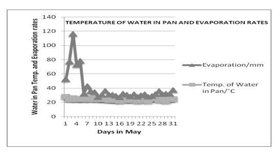
Figure 6: Temperature effect on evaporation
