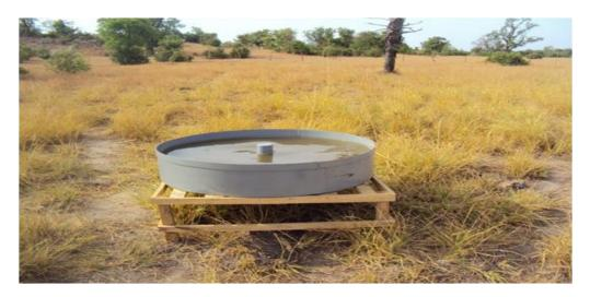
Figure 2: Installed Class A Evaporation pan at Dam Site
