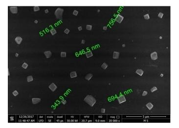
Figure 3: SEM image of the prepared nanoparticles of titanium metal
