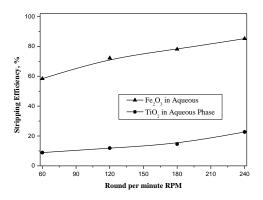
Figure 1: Effect of RPM on stripping of iron and titanium in aqueous phase.
