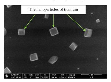
Figure 2: SEM image of the prepared decahedral nanoparticles (646.5 nm) of titanium metal
