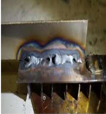
Figure 1A, 1B: Pore occurring after weld [5],
