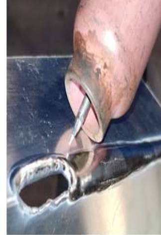
Figure 1C: Weld explode after TIG welding [6]
