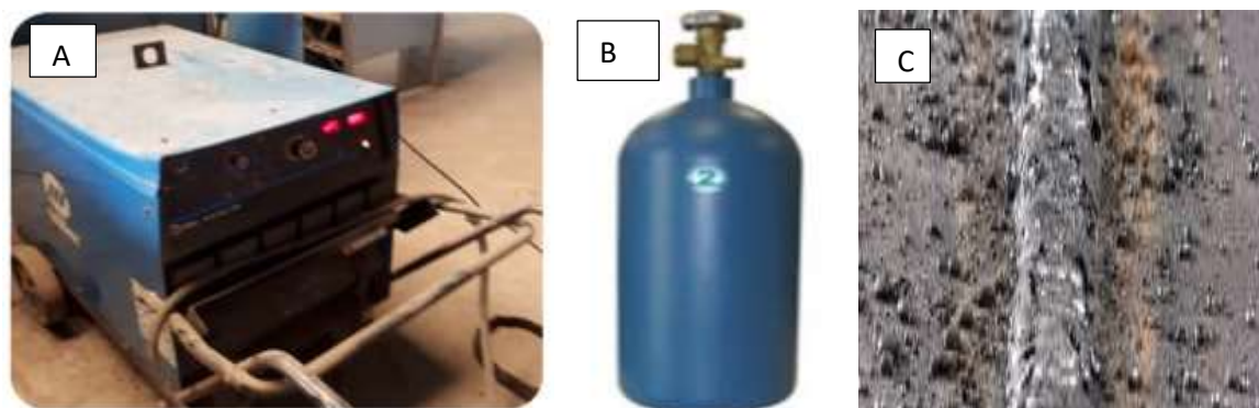
Figure 2: (A) TIG equipment (B) Shielding gas cylinder and regulator (C) Spatter images
