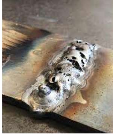
Figure 1C: Weld explode after TIG welding [6]
