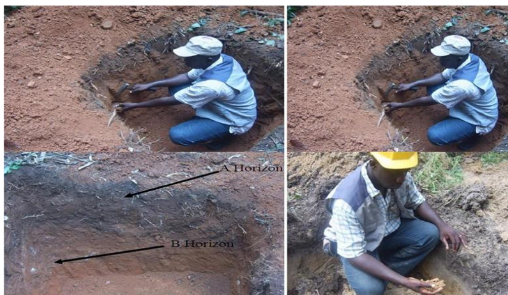
Figure 13. Pit profile showing the soil horizons up to 1.0 m depth.
