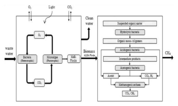
**Figure 3:** Microalga-bacterial wastewater treatment and the biogas production process **Source**: Wieczorek, Nils, Mehmet Ali Kucuker and Kerstin Kuchta. "Microalgae-Bacteria Flocs (MaB-Flocs) as a Substrate for Fermentative Biogas Production." *Bioresource Technology Journal* 194 (2015): 130 – 136. Print. Figure 3.
