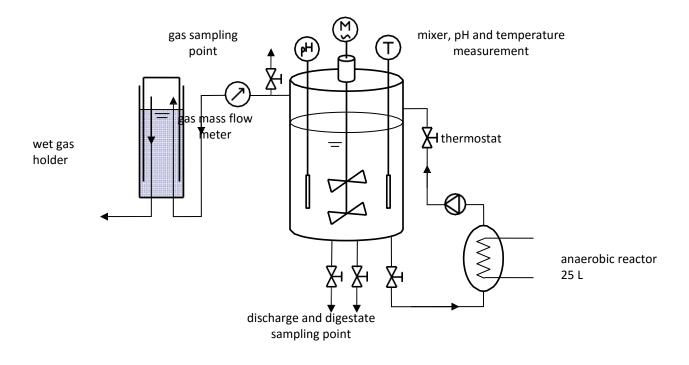
**Figure 2:** Schematic representation of an anaerobic digestion pilot plant as used in the laboratory **Source:** Stritesky, Lubos et al. "Biogas Production from Algal Biomass from Municipal Wastewater Treatment". *Symbiosis International Conference* (2014): 1 – 6. Print. Figure 1.
