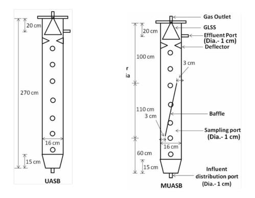
**Figure 5:** Schematic representation of UASB and MUASB reactors **Source**: Das, Suprotim and Chaudhari, Sanjeev. "Effect of Reactor Configuration on Performance during Anaerobic Treatment of low strength Wastewater." *Environmental Technology Journal* 36:18 (2015): 2312 – 2318. Print. Figure 1.
