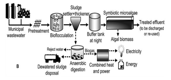
**Figure 1:** Schematic representation of a municipal wastewater treatment plant **Source:** Khiewwijit, Rungnapha et al. "Energy and Nutrient Recovery for Municipal Wastewater Treatment: How to Design a feasible Plant Layout?" *Environmental Modeling and Software Journal 68* (2015): 156 – 165. Print. Figure 2b.
