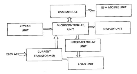
Figure 1: Block diagram of an arm-cortex based energy prepaid meter
