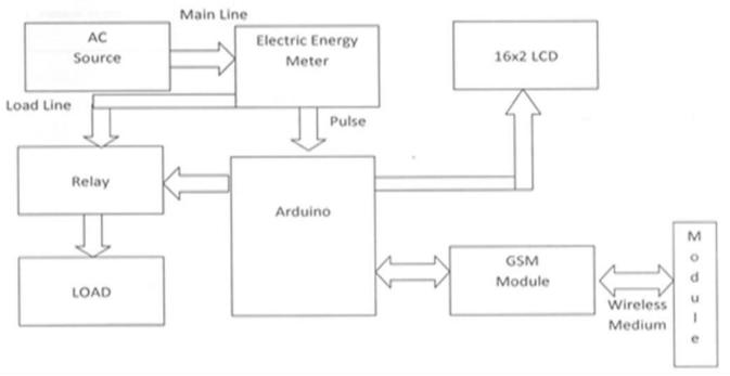
Figure 2: Block diagram of energy prepaid meter using GSM and Arduino
