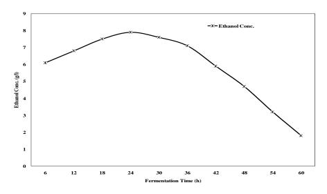
Figure 3. Effect of fermentation time on ethanol concentration
