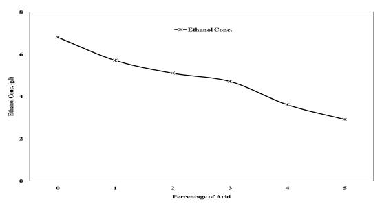
Figure 1. Effect of acid on ethanol concentration
