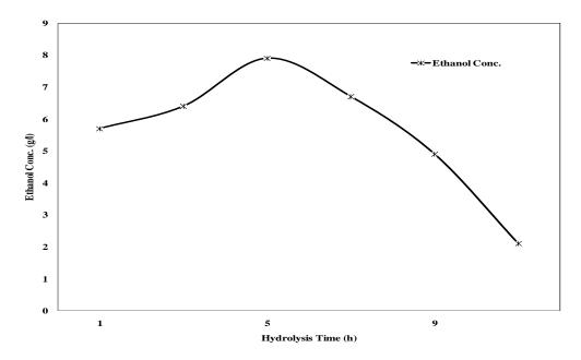
Figure 2. Effect of hydrolysis time on ethanol concentration
