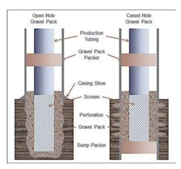
Figure 1: Internal Gravel Packing [13]
