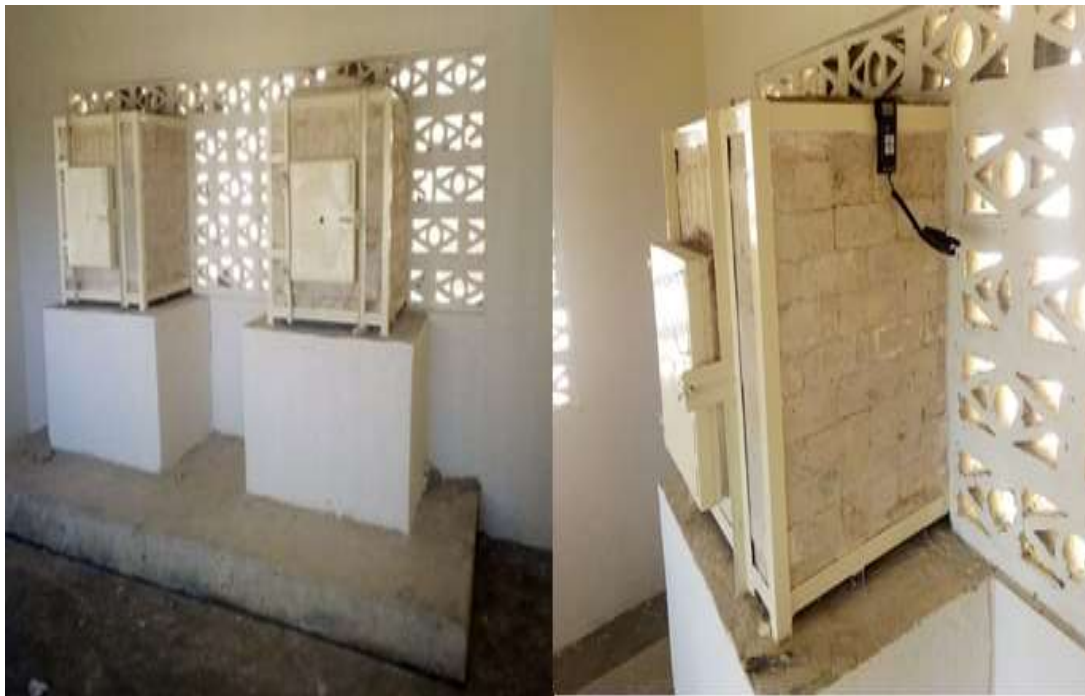
Fabricated furnace and Annealing Section
