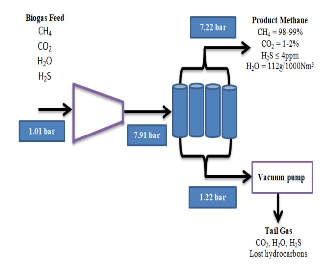
Figure 3: The process and flow during the biogas treatment.
