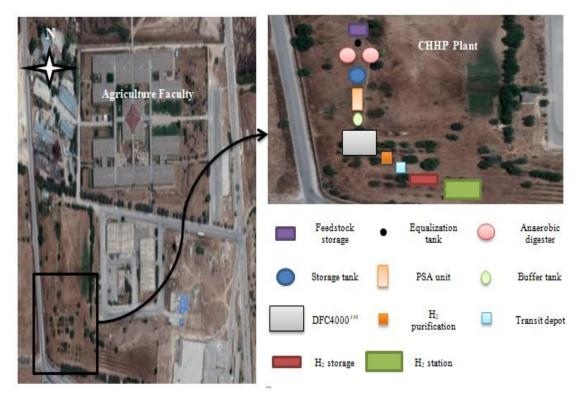
Figure1: Location with anaerobic digester, CHHP plant, and hydrogen fueling station.
