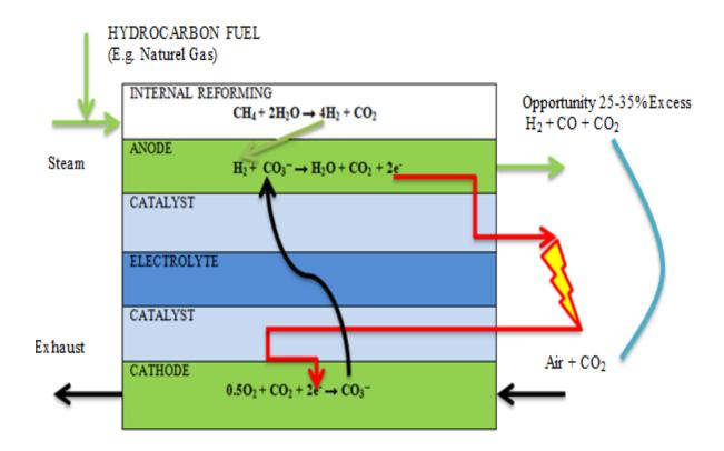
Figure 4: Internal reforming DFC<sup>®</sup> technology.
