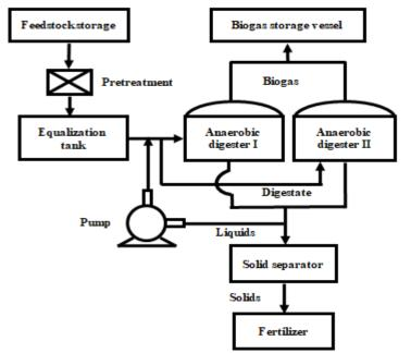
Figure 2: Flow diagram for digester and biogas production.
