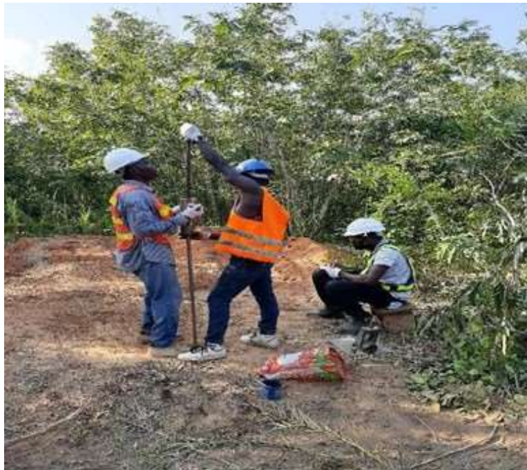
Figure 3.2: Sinking of DCP 1 at the site
