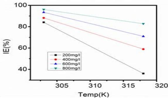
Figure 9: Gravimetrically determined I E against temperature
