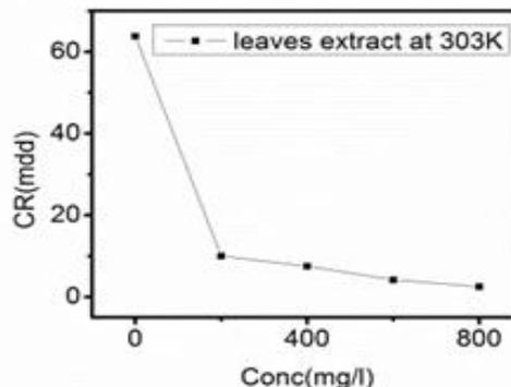
**Figure 1:** Gravimetrically determined CR against conc. at 303K.
