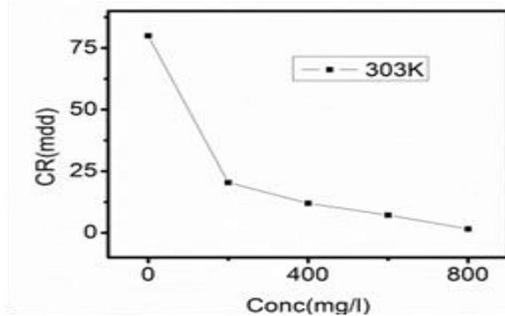
Figure 4: Gasometrically determined CR against conc. at 303K.
