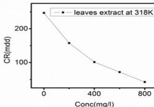
**Figure 2:** Gravimetrically determined CR against conc. at 318K.
