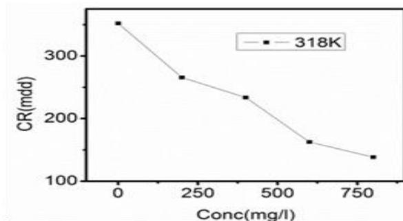
Figure 5: Gasometrically determined CR against conc. at 318K
