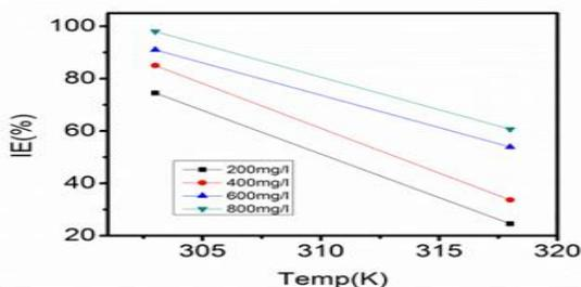
Figure 10: Gasometrically determined I E against temperature
