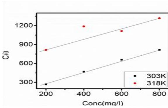
Figure 8: Gasometrically determined Langmuir Isotherm.
