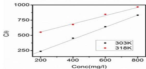
Figure 7: Gravimetrically determined Langmuir Isotherm
