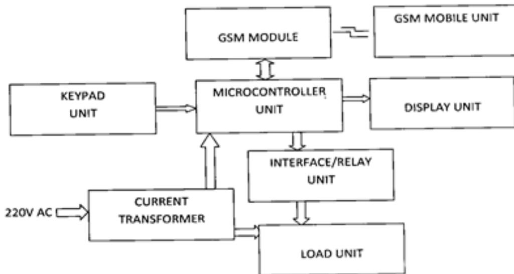
**Figure 1:** Block diagram of an arm-cortex based energy prepaid meter
