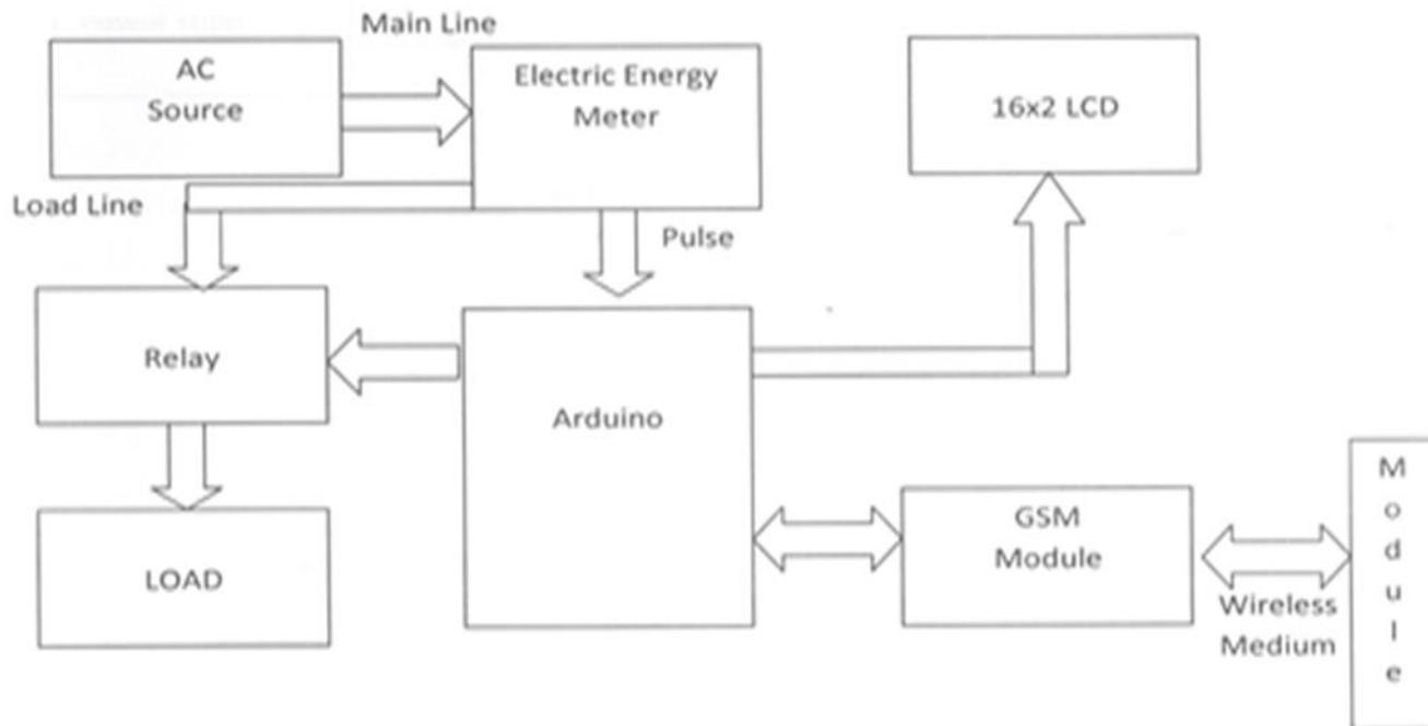
**Figure 2:** Block diagram of energy prepaid meter using GSM and Arduino
